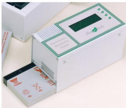
**Fig. 1-4.** Inserting the battery into the FMS2.
