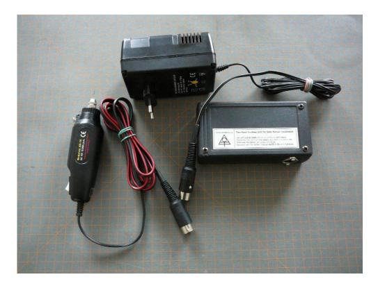
It consists of the drill, battery box with electronics and battery charger. The drill keeps low revolutions until it faces a hard xylem. Then, it increases the power until
