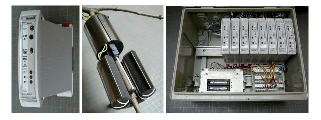
The module is supplied with 11 to 16 V D.C. The power consumption is proportional to the sap flow rate and it ranges between ca 20 and 150 mA. Output signal voltage is proportional to the heating power and it can be directly measured or registered by any common datalogger.
