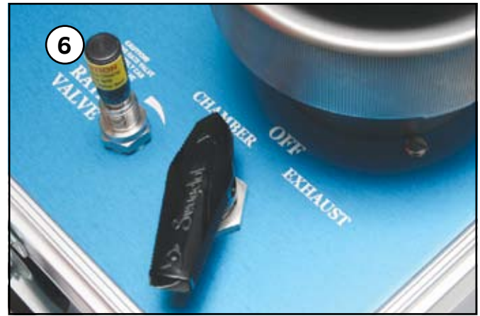
Begin to slowly apply pressure to the chamber
