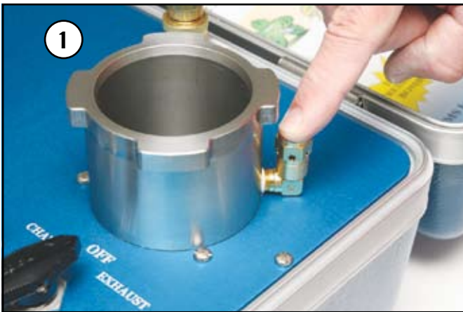
First, use your finger to depress the piston so that it is inside the safety valve
