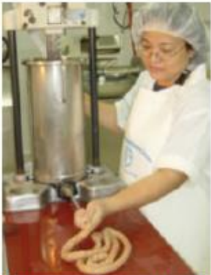
Step 5: Sausage stuffing (manual stuffer)
