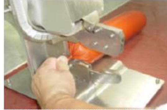
Step 9 : The sausage end is sealed using a metal clip
