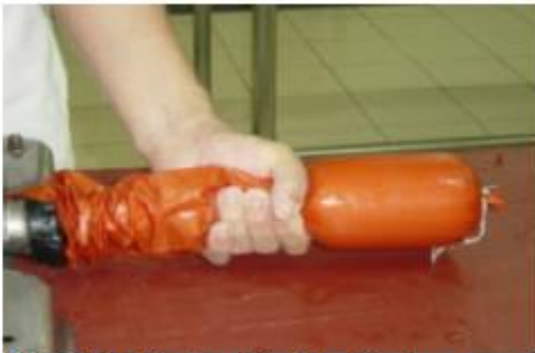
Step 8 : Product is filled into an individual casing of larger calibre
